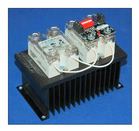
4-20MA LOOP POWERED BURST FIRING MODULE
