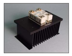
Heat Sink Dimensions: 5.25" x 3.0" x 2.75" Overall size w/Single SSR and Touch Safe Cover & DIN Clip: 5.25" x 3.0" x 4.25" Anacon's "Cool One" heat sink designs provide a thermally optimized Panel mounting platform for today's high performance solid state relays. The listings below provide the actual load currents that each part type will support. If you're not sure about how to select the correct product for your application, call Anacon, toll free and discuss your application with us.
